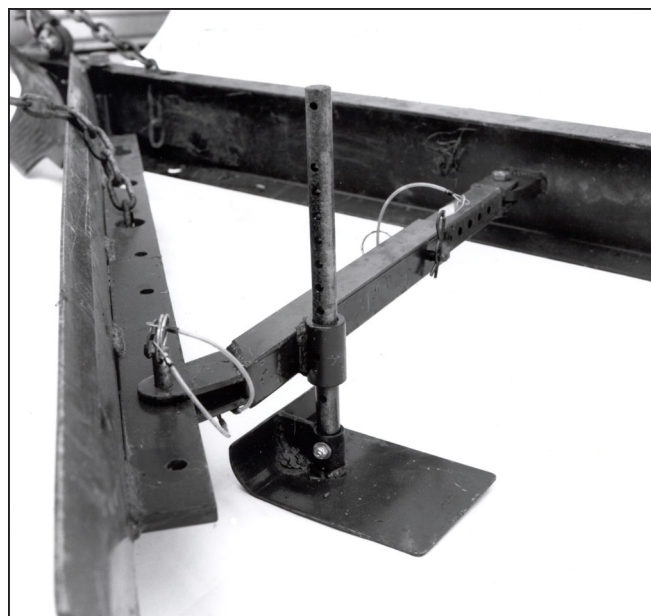
Figure 26—Shoe and wing adjustments of the MTDC combination plow and grader.
