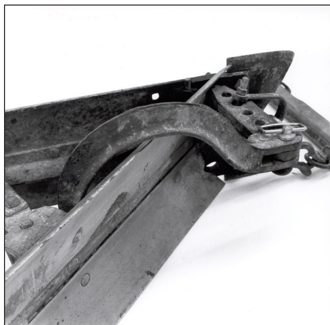
Figure 21—Closeup of Beatty trail grader hitchbar and wing.
