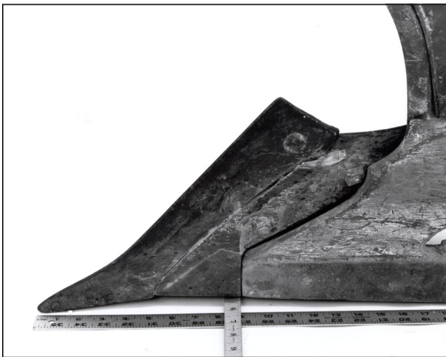
Figure 11—Oliver plow showing about \frac{3}{14} inch of bottom suction.
