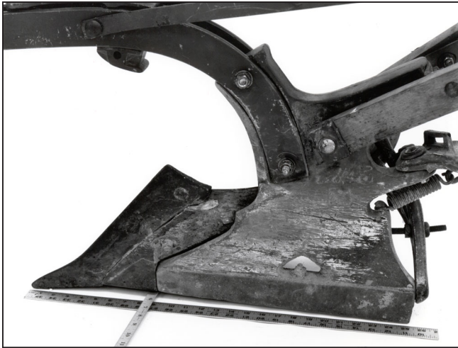
Figure 10—Oliver plow showing about \frac{1}{12} inch of hillside suction.
