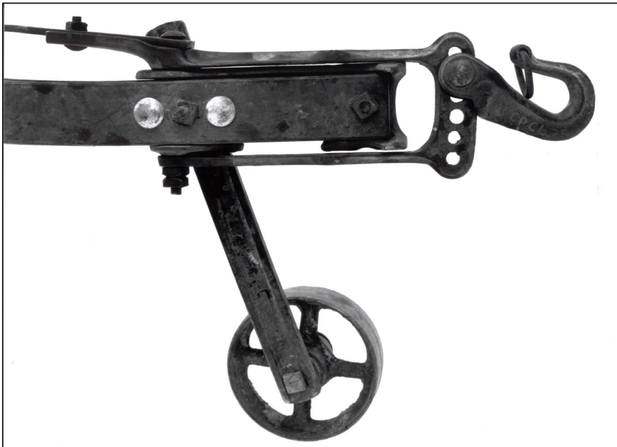
Figure 3—Vertical draft adjustment.
