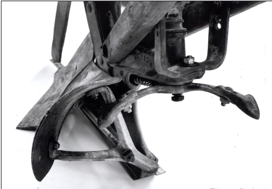
Figure 2—The latch on a hillside plow.
