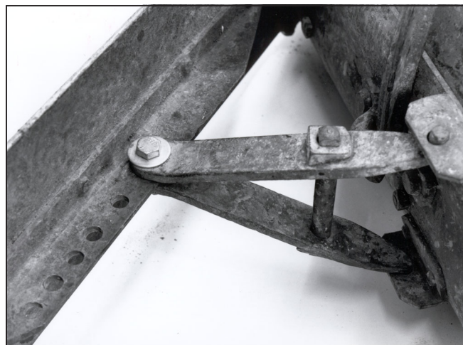
Figure 22—Beatty trail grader wing adjustment.
