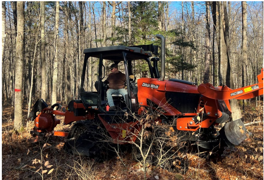
Trenching an oak wilt pocket in Pigeon River with a vibratory plow Country.
