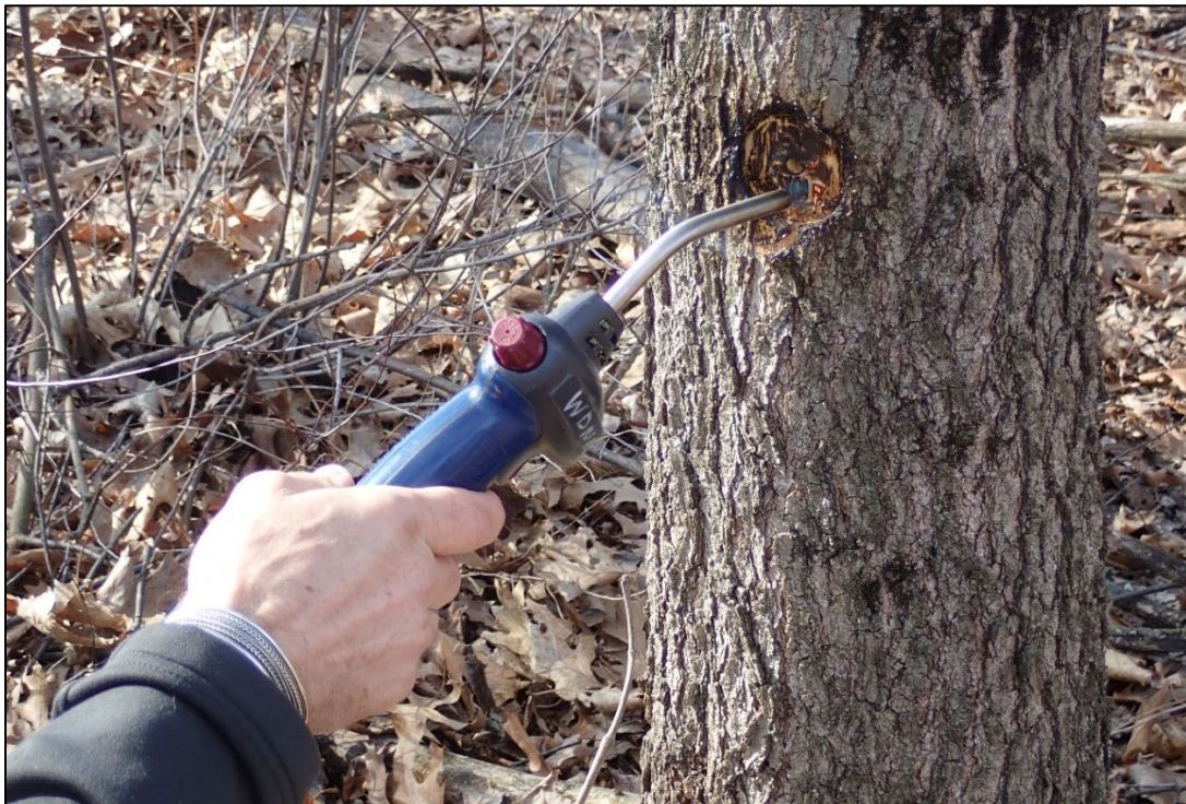
Figure 32. Simulating a fire wound with a propane torch. / Photo Credit: Wisconsin DNR
