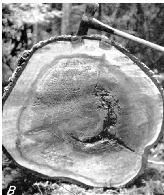
Figure 2.—Typical brown rots in western hemlock: A, Shattered log showing longitudinal view of advanced decay in the heartwood caused by the velvet top fungus; B, cross section of a log showing advanced and incipient stages of decay caused by the sulfur fungus; C, tangential section of advanced decay (above) and radial section (below) showing advanced and incipient stages of decay caused by the red belt fungus.
