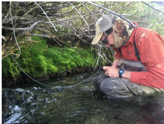
Figure 27. American Conservation Experience intern with the hydrology crew installing temperature loggers in Colorado River cutthroat trout habitat as part of Focal Species Monitoring Program (2019).
