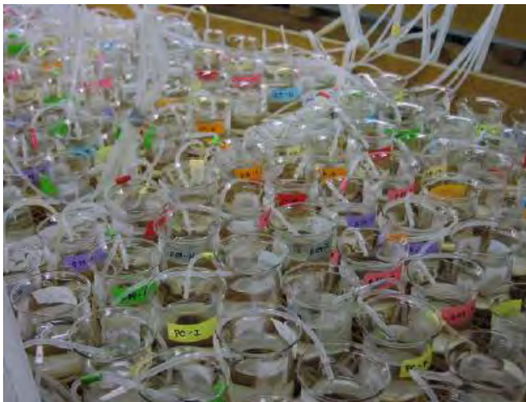
Figure 3. Chronic trout test setup (top) and chronic midge test setup (bottom). Photos from McKee and Hansen (2005).
