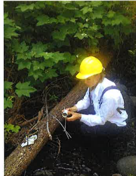
Figure 2. Installation of a stream temperature logger
