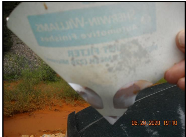
Photo 14. Successful paint filter test (No water!)
