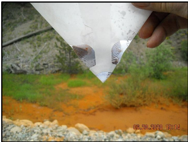
Photo 15. Successful paint filter test (No water!)
