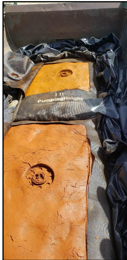
Photo 17. Dewatered and densified sludge
