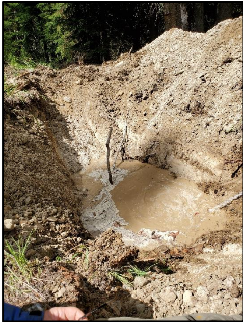
Photo 18. Infiltration test, BLK-TP2
