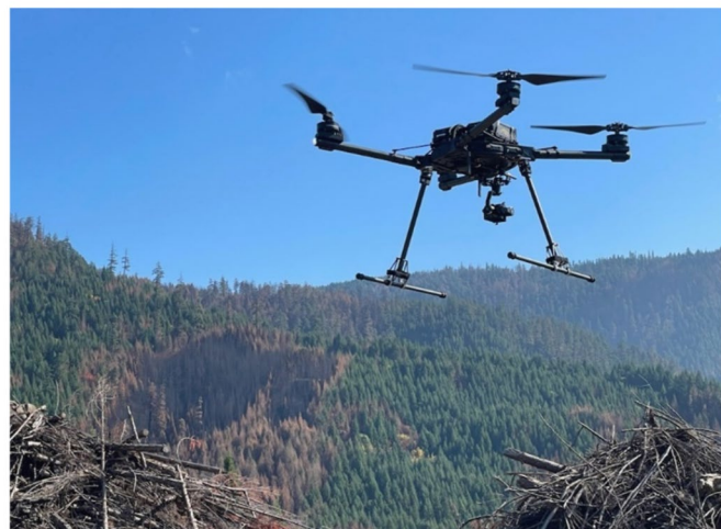
Behind the Uncrewed Aerial System (UAS), the Chilcoot Fire's perimeter can be seen. This UAS flew a reconnaissance mission along the western flank's perimeter to detect heat using an infrared camera. USDA Forest Service Photo.
