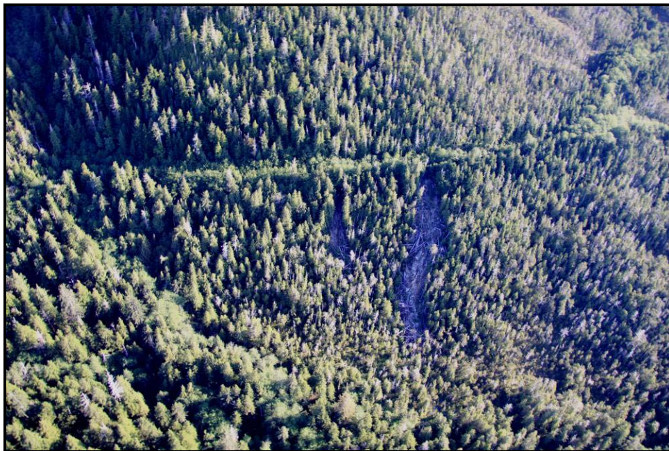
Figure 4-38. Aerial photo looking north across the OSA-300 haul road showing the east (right) and west landslides that are located approximately 700 feet east of the 300-Foot Level
