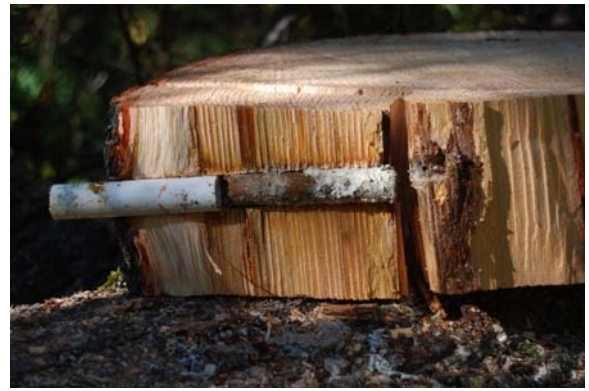
Fig. 2 – An inoculated trunk section of a sampled Douglas-fir. Note the white mycelium on the colonized dowel (right) and the plastic pipe inserted partway into the drilled hole (left). Only a small amount of decay is shown here that is associated with the colonized dowel after 10 years.
