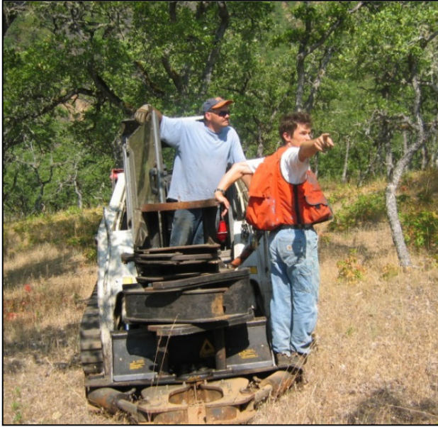
The Lightfoot™, Integrated Resource Management's lightweight machine used for harvesting small-diameter stems and masticating brush.
