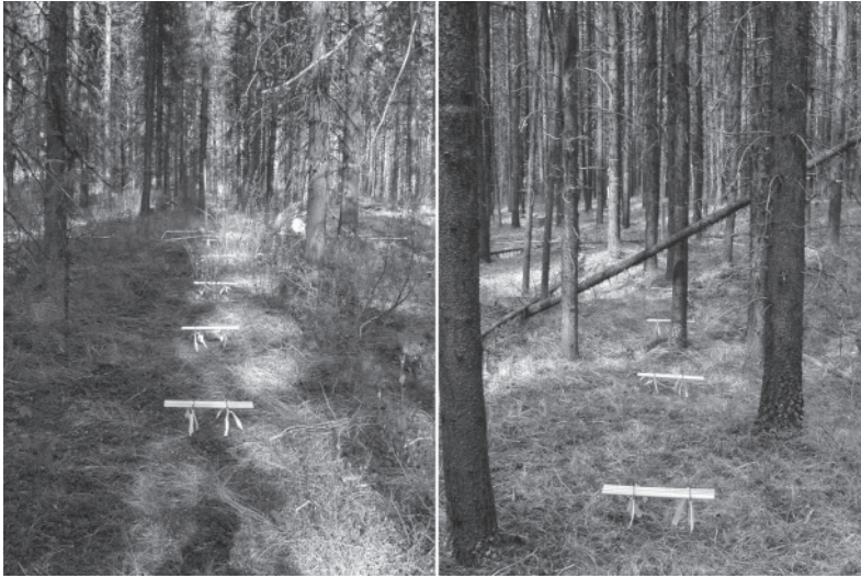
Figure 2 —Five sets of fuel moisture sticks set up in the thinned stand (left) and in the control stand (right).
