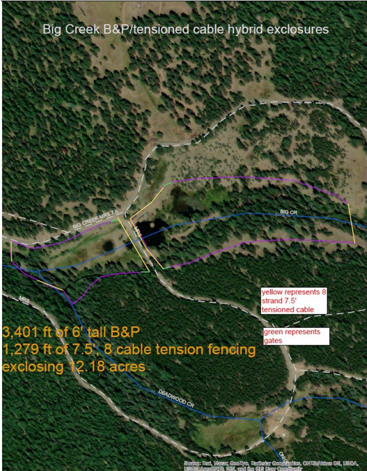
Figure 5. Big Creek exclosure, tensioned cable and buck and pole design. Purple represents buck and pole fencing.
