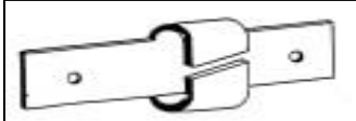
Figure 7. Metal Clip. Excellent on either wood or steel posts. Easy to install, no maintenance and allows fastest wire adjustment. Existing fences easy to modify with this clip. Variations of clip available for both adjustable and/or lay-down.
