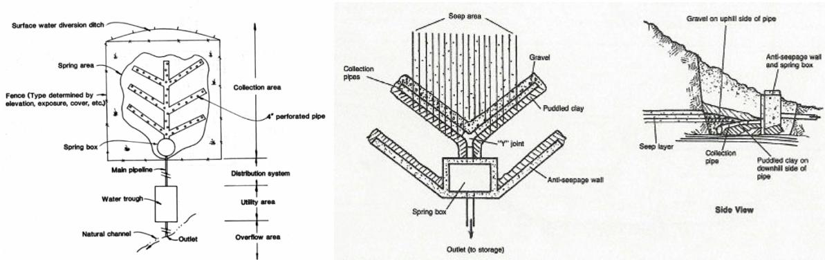
Each spring development depends on the water source, rate of flow, and the quantity of water needed, as well as available forage, slope, ecosystem, proximity to roads, wildlife use, and accessibility to equipment. The water collection system is usually protected with either wire fencing or brush fence. The water is piped from the spring source to the water trough, underground. The overflow flow the water trough is piped underground back to the natural channel.
