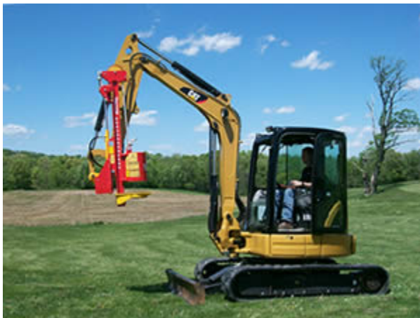
Figure 7 Mini-excavator with post pounder adapter
