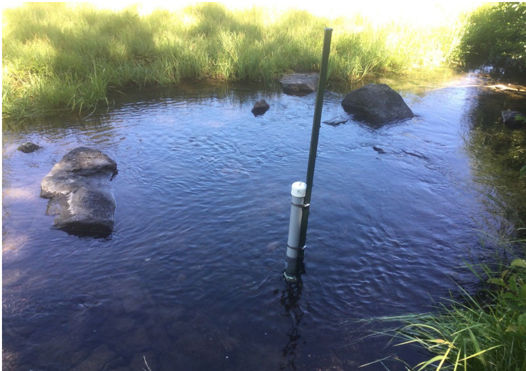
Figure 15. Example of a stream gauge installed below the Summit Creek Phase 1 project area. A "level logger" is placed within the pipe to provide continuous surface water (and thus discharge) data at the site.
