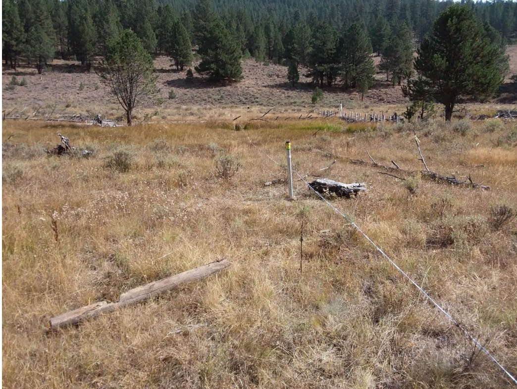
Figure 14. Example of a piezometer installed within the Summit Creek Phase 1 stage 0 project area. A "level logger" is placed within the well to provide continuous groundwater level data at the site.
