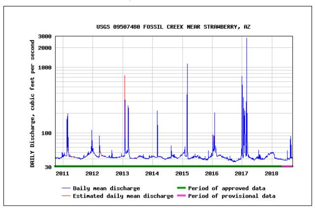
Figure 3-6. Daily mean discharge in cubic feet per second (cfs) for Fossil Creek at USGS gage 09507480
