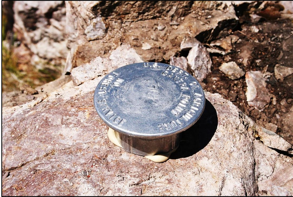
Figure 21 – Replacement camera point marker (aluminum cap) for camera point 4.
