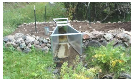
Figure 13.2. Flume gauging station on Redondo Creek
