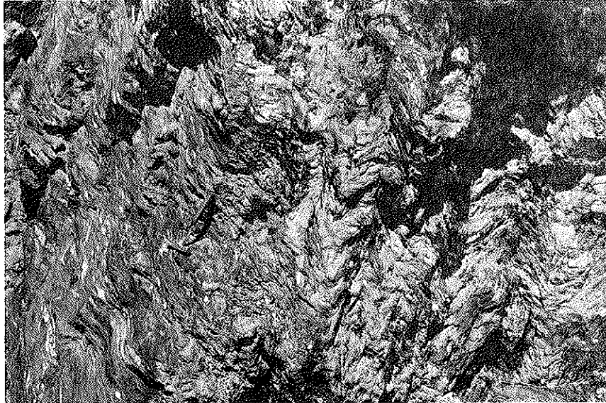
Figure 58. High grade Schist bedrock. This bedrock is intensely folded but generally hard and competent.
