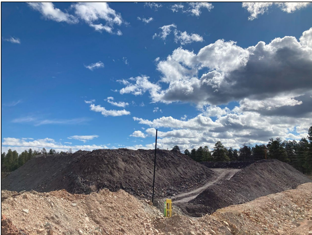
Photo 20 – Overlooking the ore pad, facing NE. Pole is used to determine height of stockpile. (Apr. 29)
