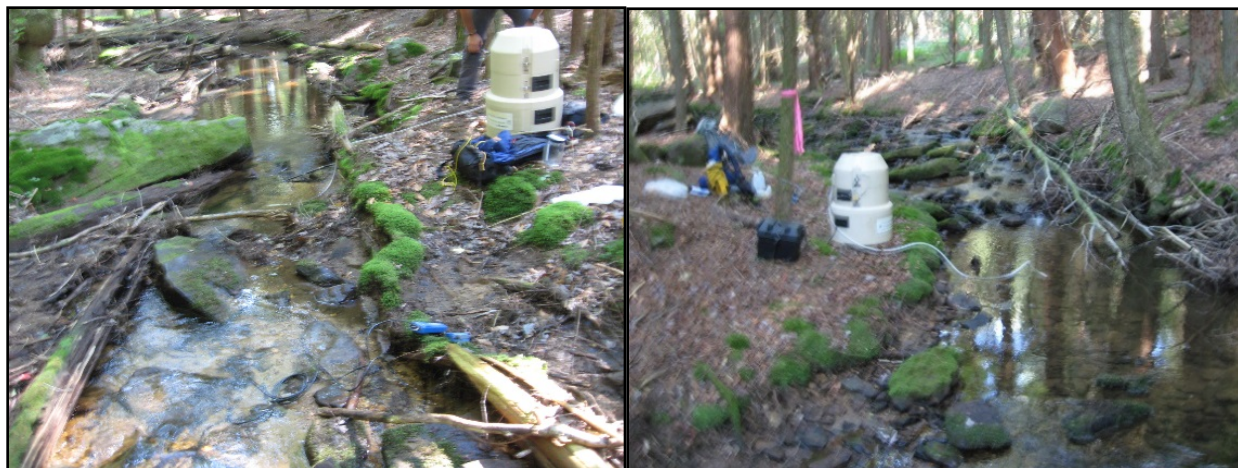
Figure 50. American Sigma® Model 900 automatic samplers at control and treatment sites on Little Arnot Run
