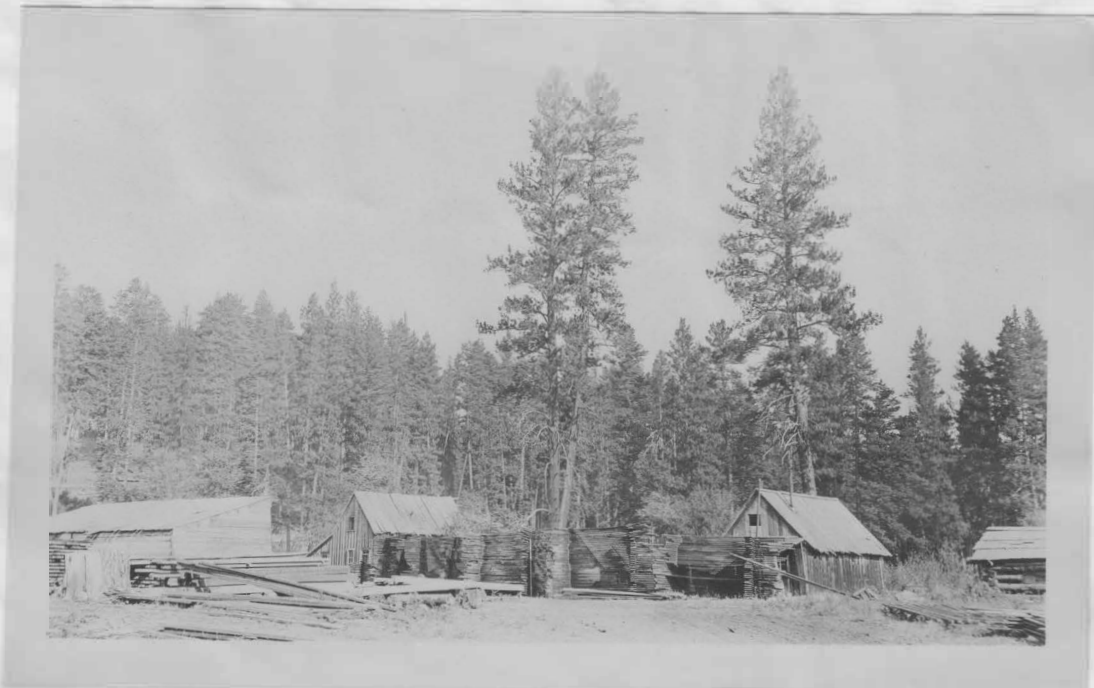
No. 18. Lumber racked for drying, also showing dry shed, owner's house and bunkhouse.
