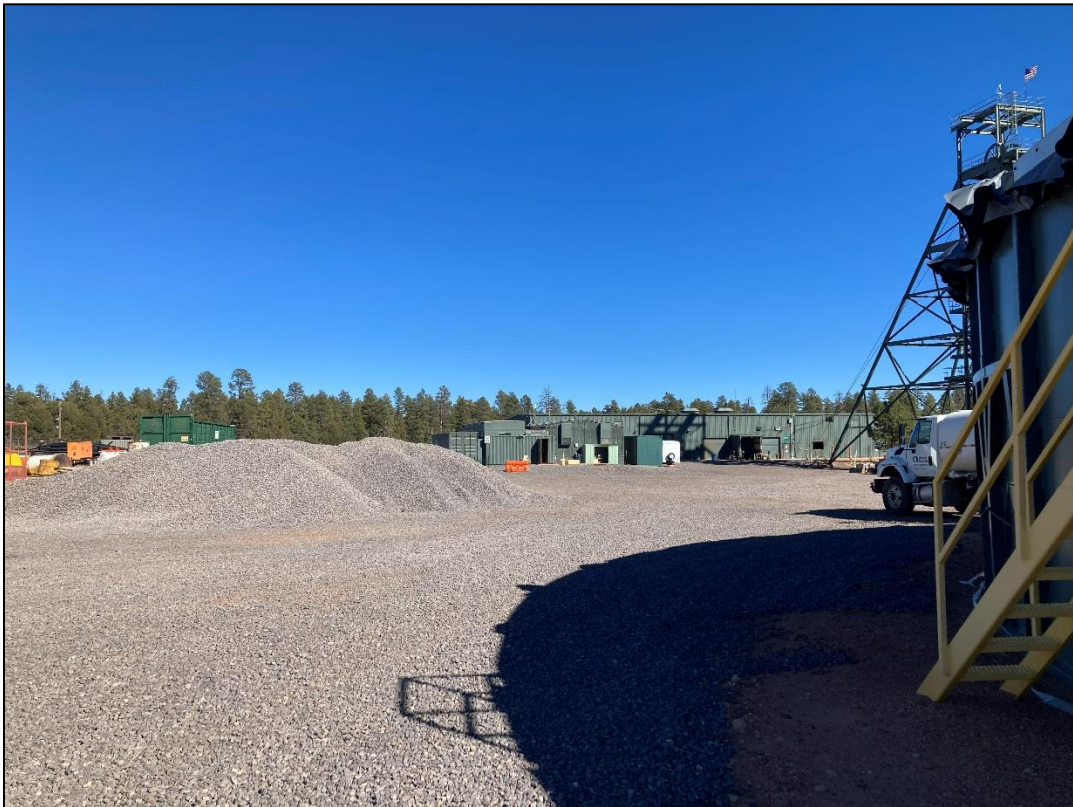
Photo 6 – Gravel stockpile used to reinforce pathways within the perimeter of the mine. (Nov. 25)
