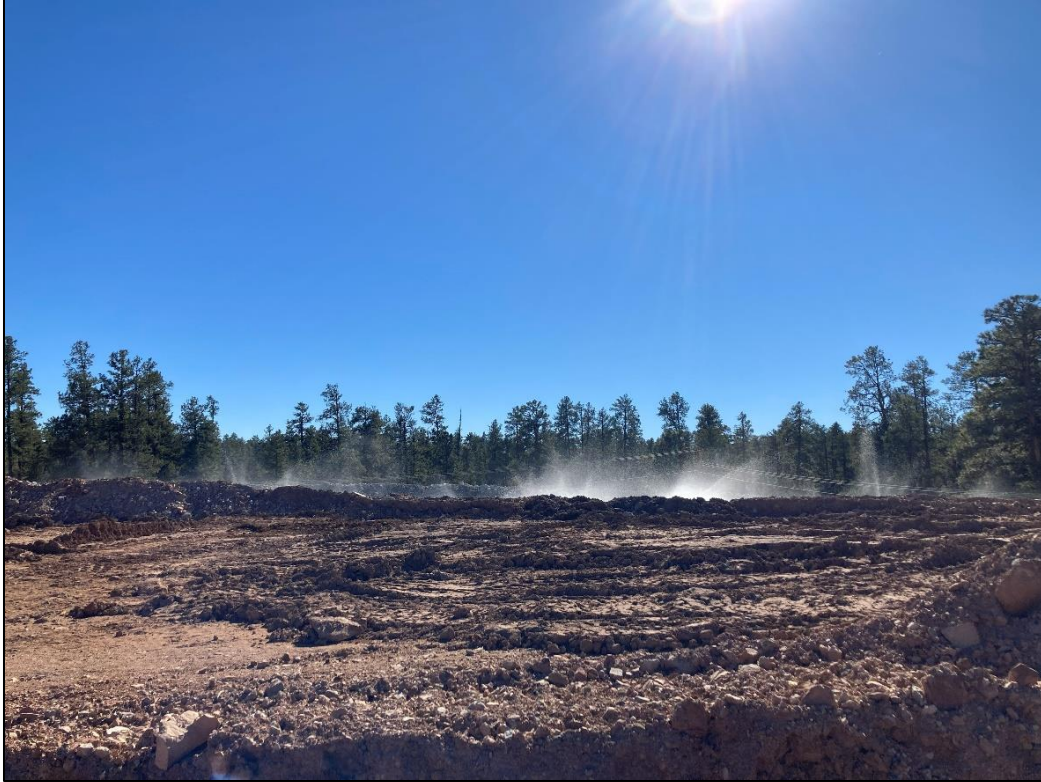
Photo 17 – Overlooking upper surface of development rock stockpile, facing south. Hoses were online for dust abatement during site visit. (Oct. 28)
