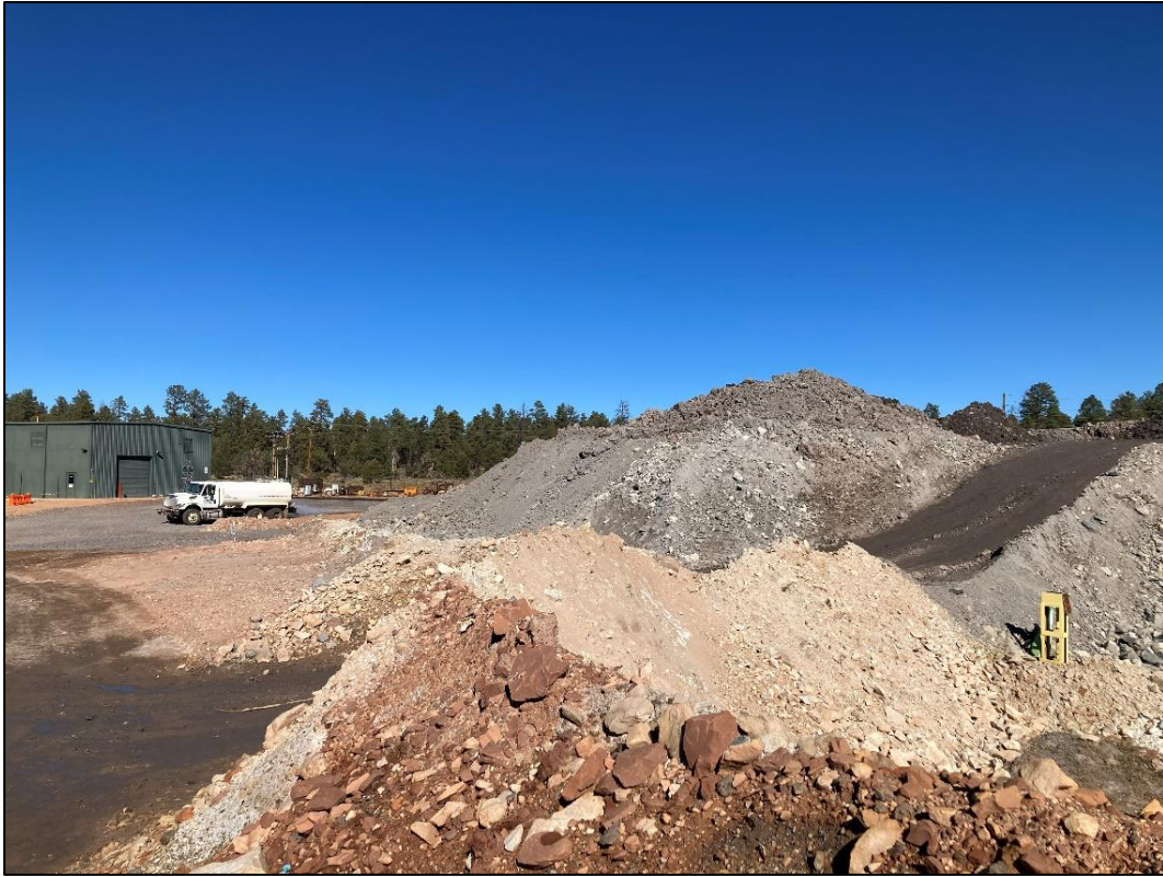
Photo 20 – Ore stockpile. Water tender was used on stockpile ramps for dust abatement. (Oct. 28)
