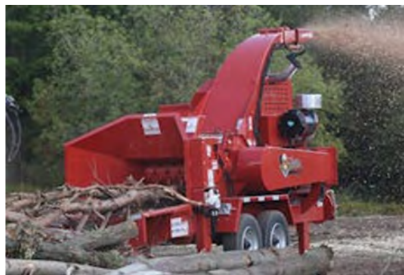
Figure 11: Examples of a mowing attachment (left) and a pull-behind chipper (right). Mowers such as the brush hog mower shown above can be pulled beside or behind a tractor and may be used to treat brush species or grasses. Chippers produce chips of vegetation, operated by a crew of people or by remote, and may be pulled behind a vehicle as the one pictured above or operated with controls on tracks in a variety of equipment configurations (image sources: left- https://bushhog.com/full-product-guide/ ; right- https://www.morbark.com/product/m20r-forestry-whole-tree-drum-chipper/ ).
