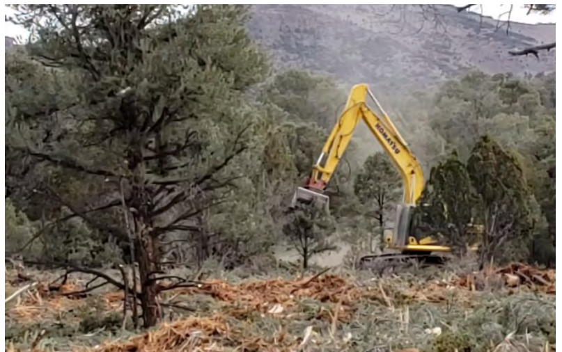
Figure 2: Masticators like those shown above shred and chip vegetation in a similar manner to brush saws. Masticator heads can be attached to different types of equipment with different sizes and capabilities. Often excavator-base tracked equipment with a boom arm and masticator attachment is the preferred piece of equipment due to its low pressure ground disturbance (<8psi) and smaller travel footprint, requiring one path to much vegetation rather than several passes that other equipment may require to produce the same result (image source: USFS).
