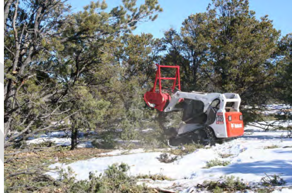
Figure 1: Two examples of different types of brush saws. Brush saws chip and shred trees and brush up to 15 feet tall. Brush saws have a variety of cutting heads that can attach to several different pieces of equipment as shown above (image source: https://revegetation.greatbasinfirescience.org/equipment/hydraulic-shearing-blades-and-brush-saws/ ).
