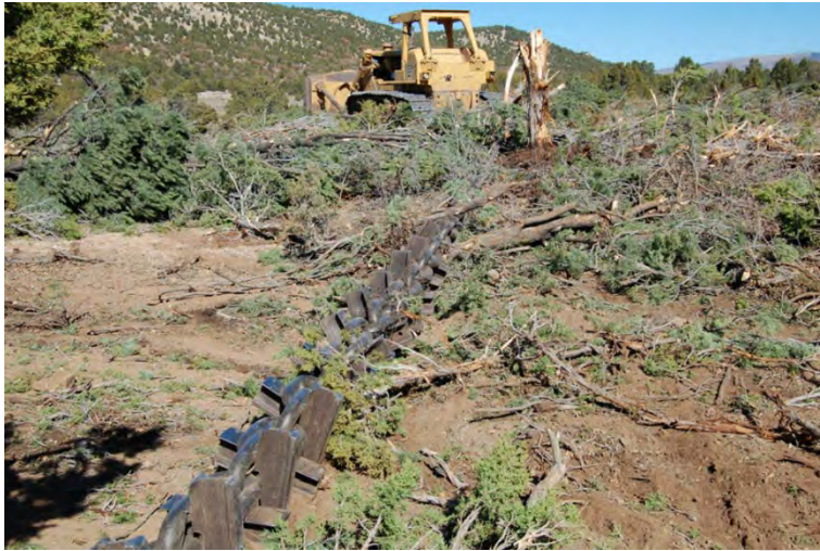
Figure 6: Chaining uses a large anchor chain dragged between two dozers to rearrange vegetation. Chaining can be done with a smooth chain (often chosen for reseeding in fire burned areas to restore native vegetation) or an Ely anchor chain (shown above- uproots pinyon and juniper trees, leaving clear ground for newly seeded grasses and shrubs to grow) with different methods depending on objective of the treatment. Chaining provides openings in the soil that are receptive to seeding of grasses and shrubs that occurs with this process and produce a positive vegetation response after treatment while also providing cover and habitat microclimates wildlife, (image source- USFS).
