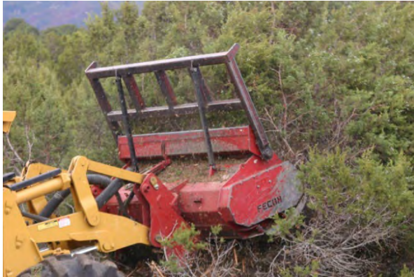
Figure 1: Two examples of different types of brush saws. Brush saws chip and shred trees and brush up to 15 feet tall. Brush saws have a variety of cutting heads that can attach to several different pieces of equipment as shown above (image source: https://revegetation.greatbasinfirescience.org/equipment/hydraulic-shearing-blades-and-brush-saws/ ).
