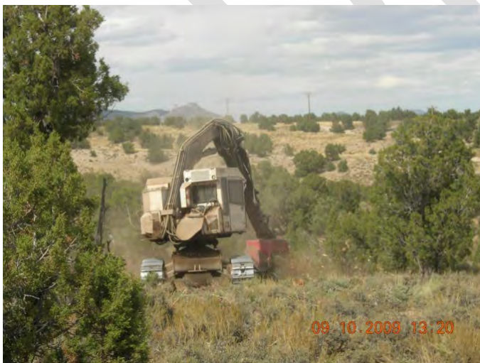
Figure 2: Masticators like those shown above shred and chip vegetation in a similar manner to brush saws. Masticator heads can be attached to different types of equipment with different sizes and capabilities. Often excavator-base tracked equipment with a boom arm and masticator attachment is the preferred piece of equipment due to its low pressure ground disturbance (<8psi) and smaller travel footprint, requiring one path to much vegetation rather than several passes that other equipment may require to produce the same result (image source: USFS).
