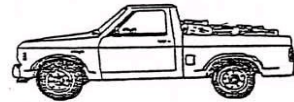
Short Bed Pickup – ½, ¾, or 1 Ton With or without racks, this truck will also hold approximately ½ cord of wood. (approx. 1331 lbs.)
