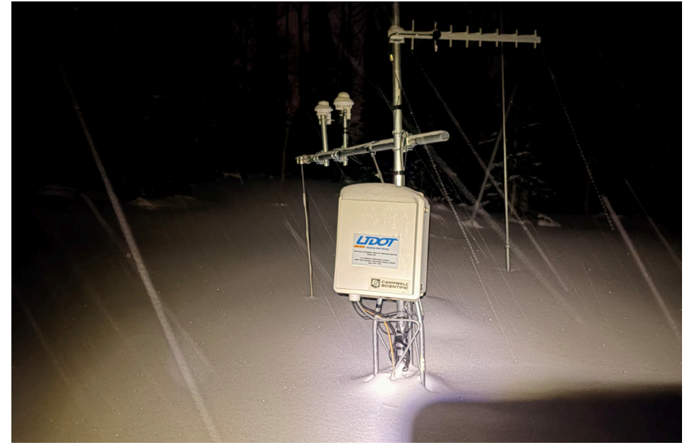
One of our research towers deployed at Atwater study plot in Alta. The atwater study plot gives us a testbed for testing new sensors, their configurations, in a representative test bed before deploying out to our other sites.
