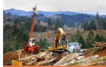
▲ Shovel yarder truck
