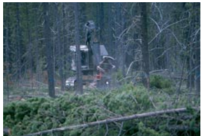
Figure 29. The feller-buncher offers a higher degree of control and safety than manual thinning and slash piling.
