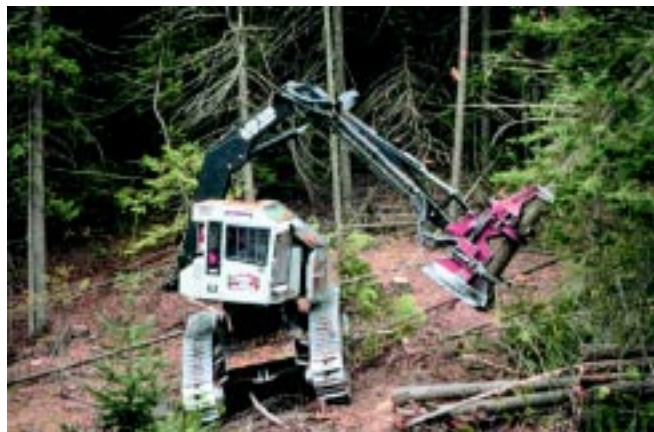
Figure 30. A feller-buncher in operation.
