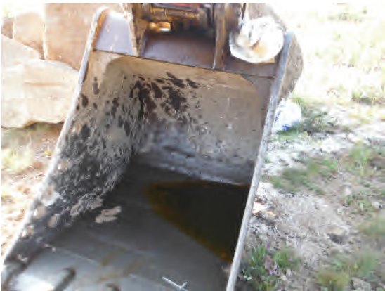
Hydraulic fluid in excavator bucket.
