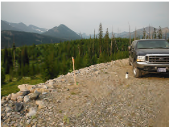
“Rocky” one of three survey control points. This is along access road south of excavation area.
