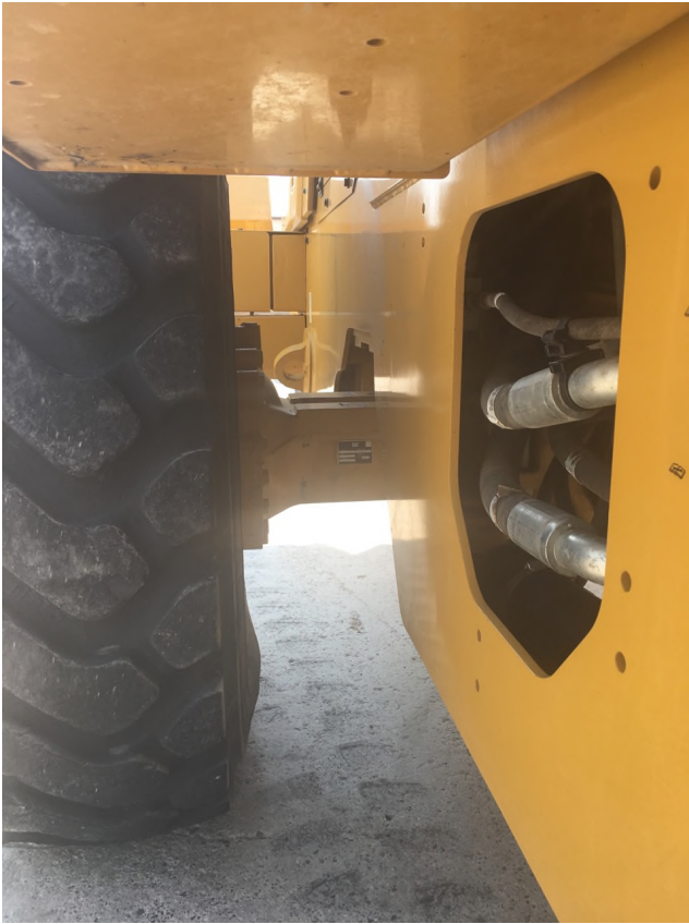
Front end loader tire and hydraulic lines
