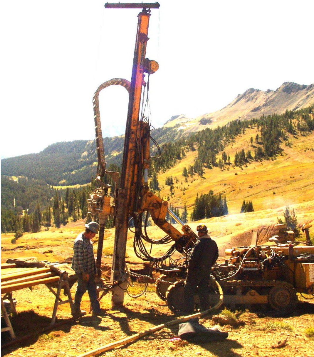
Figure 26. Rotary Drill Reaming of BQ Core Holes
