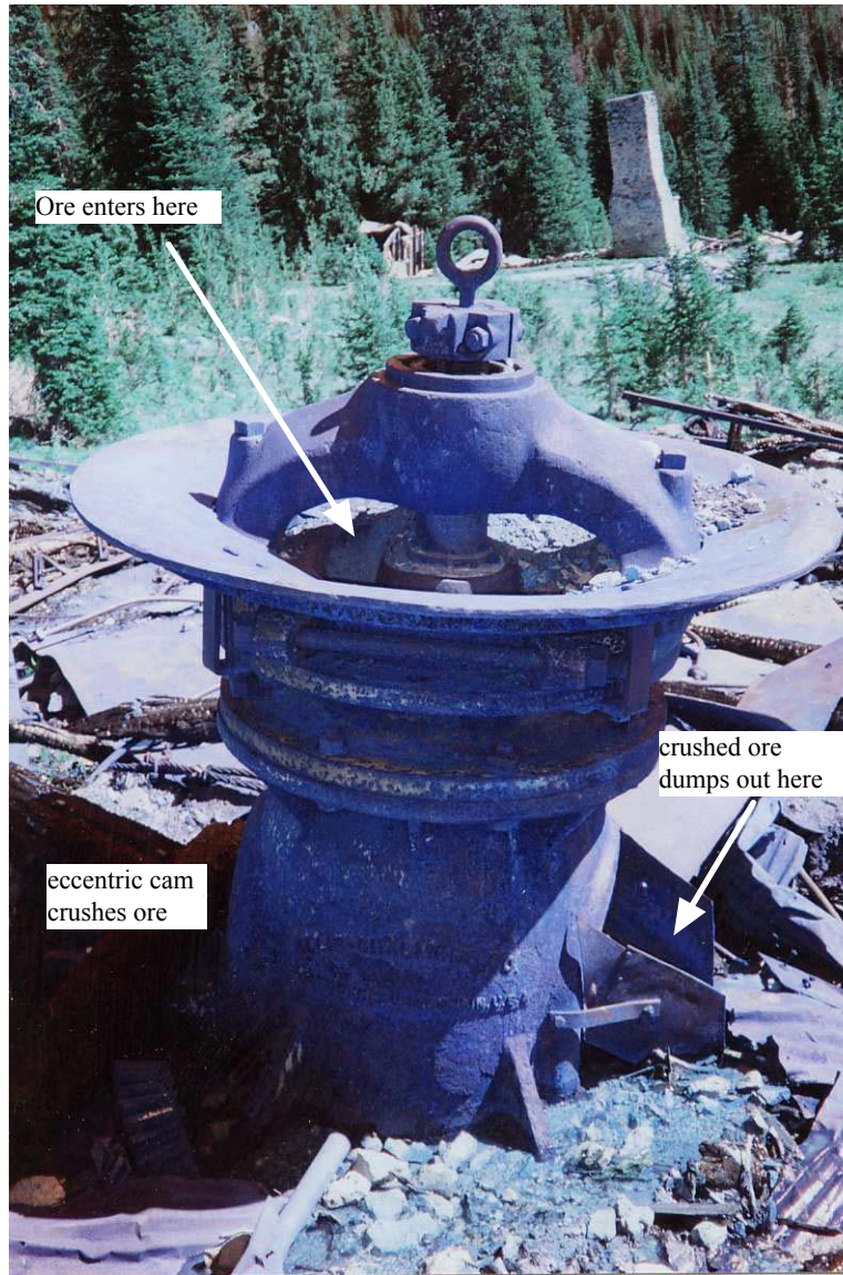
Figure 2-8. Allis Chalmers gyratory crusher at the load-out terminal of the Homestake to Gold Dust Tramway (Feature 5).
