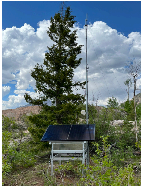
Solar panels can power device for up to 5 years
