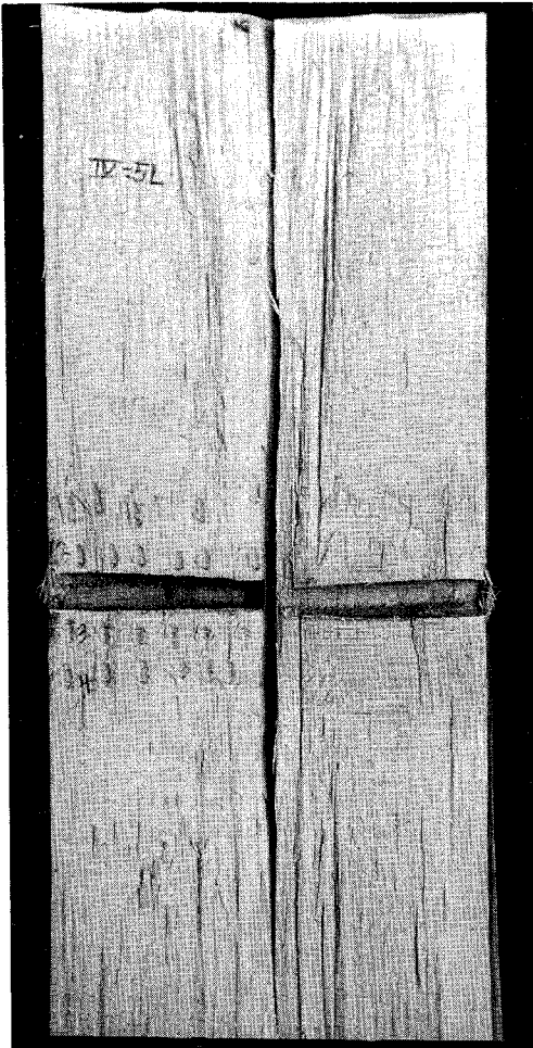
Figure 1. — Dissection of a taphole that did not receive a paraformaldehyde pill; after 60 days. The discolored area above and below the taphole was very faint and, after the wood dried, it was difficult to see the discolored area. The small holes above and below the tapholes mark the position of the chips of wood taken for isolating microorganisms.
