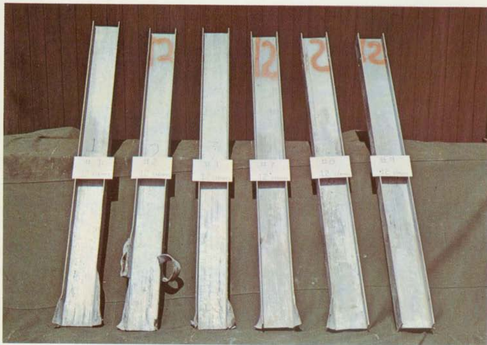
Figure 9.—Six steel posts on site 1 required 12 blows each for insertion. Damage ranged from none to severe.
