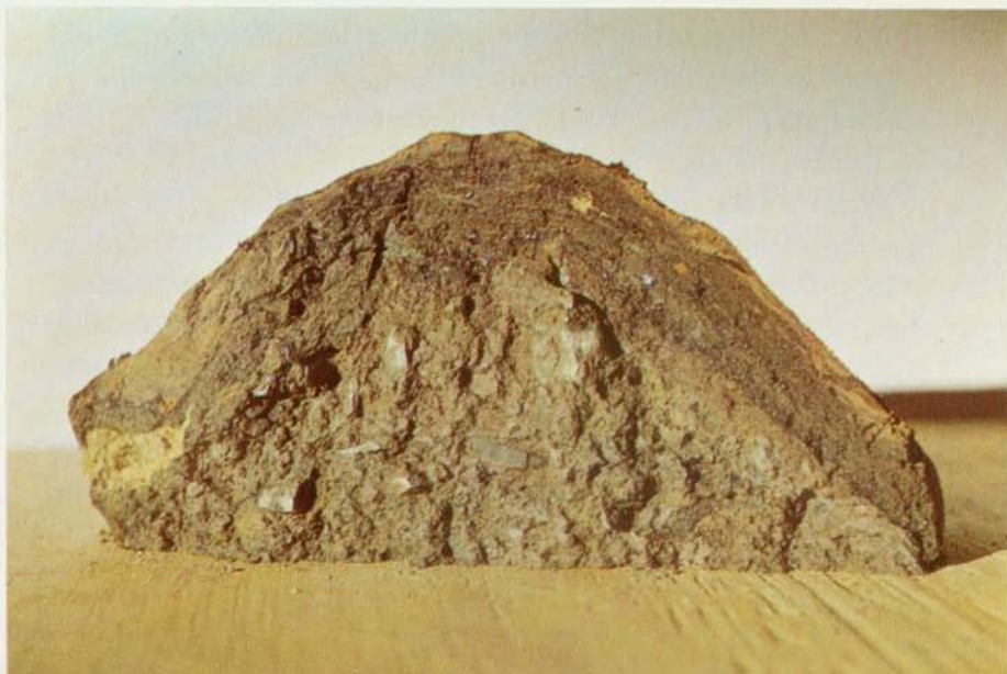
Figure 8.—Section of cone formed at the base of wooden post 16. Center of the cone is made up of limestone and shale from the top 8 inches of the site profile. In the outer inch of the cone, concentric layers of other materials can be seen.
