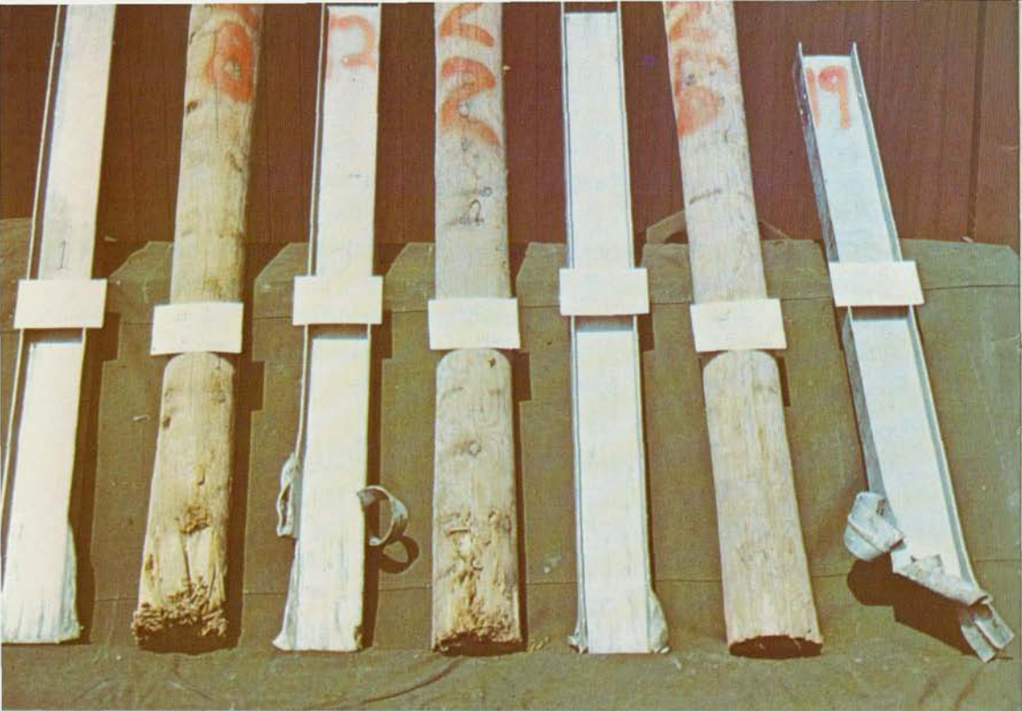
Figure 3.—The four steel posts and three wooden posts driven into the rock base of site 1. The number of blows per post with the 950-pound hammer were (from left to right): steel post 1—12 blows; wooden post 1—28 blows; steel post 2—12 blows; wooden post 2—22 blows; steel post 3—12 blows; wooden post 3—25 blows; steel post 4—19 blows.
