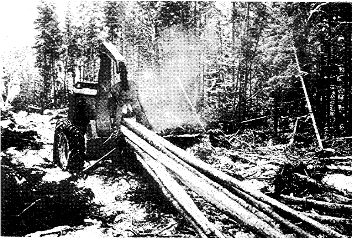
Figure 2.—A four-wheel rubber-tired skidder hauls a load of stems to a landing.
