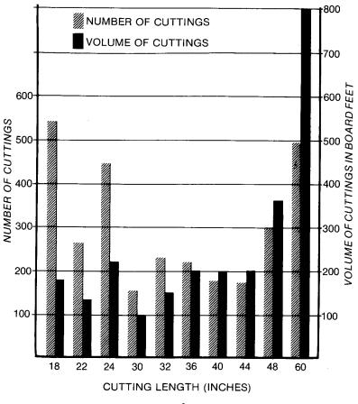
In addition to the specification of cutting sizes, the program requires input data on the location of all defects within each board. To provide these data, we collected a sample of 637 No. 2 Common 4/4 red and white oak boards and recorded the locations of all defects on them. Each defect was coded to indicate the type of defect and whether it occurred on the grade side or the back side of the board. Twenty-three defect types were recognized and recorded.
