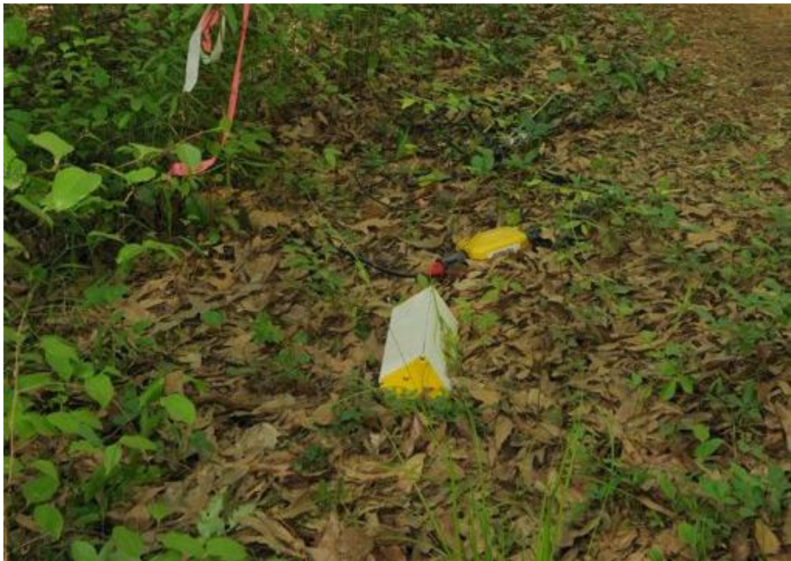
Photo 3 – Recording box and battery
