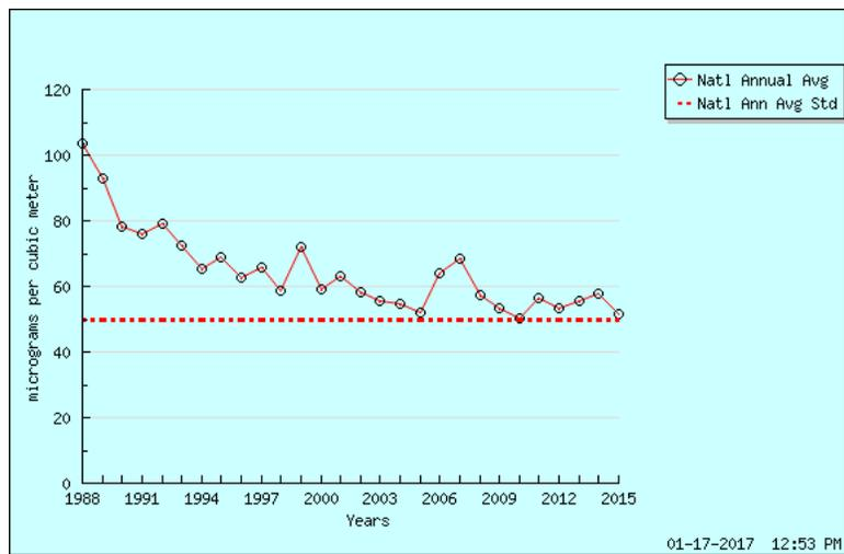
**Figure 2. The three year average PM10 trends for the South Coast Air Basin Air Basin as above the national standard of 35µg/m<sup>3</sup> since 1988. Note the graph displays the old standard – 50µg/m<sup>3</sup>.**
