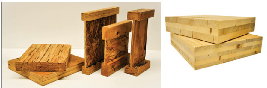
Figure 10.—Examples of engineered wood products. From left: parallel strand lumber, I-joists, and cross-laminated timber (Photo credit: Maria Fernanda Laguarda Mallo, University of Minnesota, used with permission).
