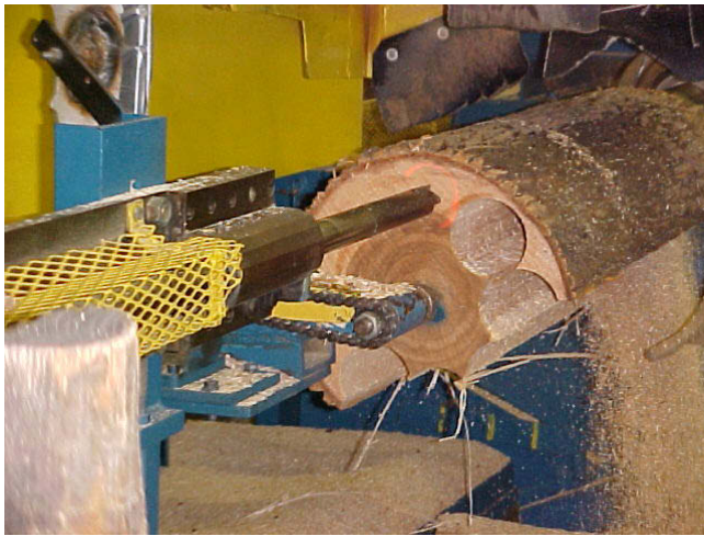
Figure 1.—Billet boring machine on which 70 percent of L&N's billets for baseball bats are produced.
