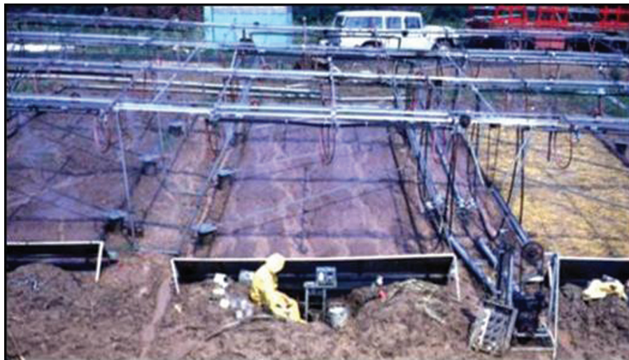
Figure 4. Standard soil erosion plots and simulated rainfall system in southern Indiana in 1968. These types of experiments were used to develop and refine the Universal Soil Loss Equation (USLE) (Photo credit: USDA Agricultural Research Service).
