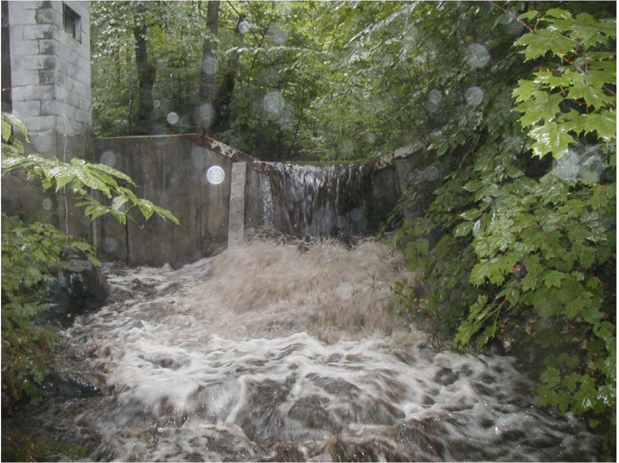
Figure S8. The W-9 gage near the peak flow response from an intense storm, 24 July 2008. Flow peaked at 476 \text{ L sec}^{-1} ( 4.23 \text{ mm hr}^{-1} ), the second highest flow recorded over about 30 years of total record at this site.
