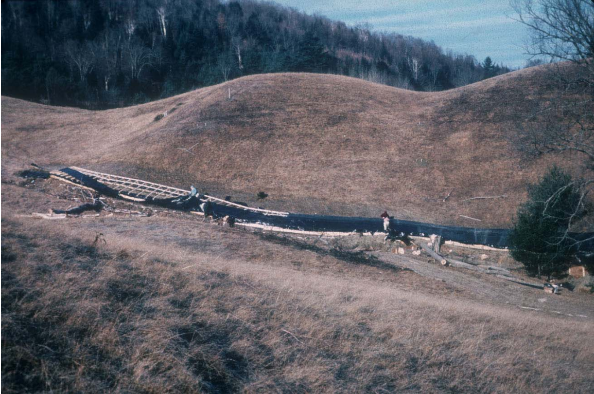
Figure S2. Dunne and Black study area (Figure 1) in the late 1960s with trench installation visible at the base of the hillslope. Note convex, concave, and planar hillslope sections.
