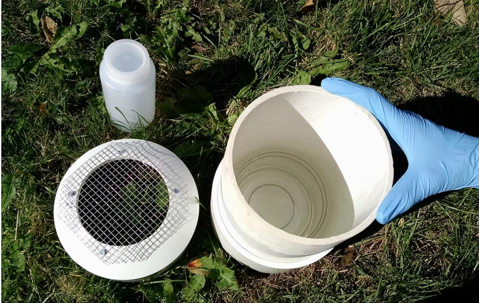
FIG 2 Photograph of the modified Tauber trap used in this study.
