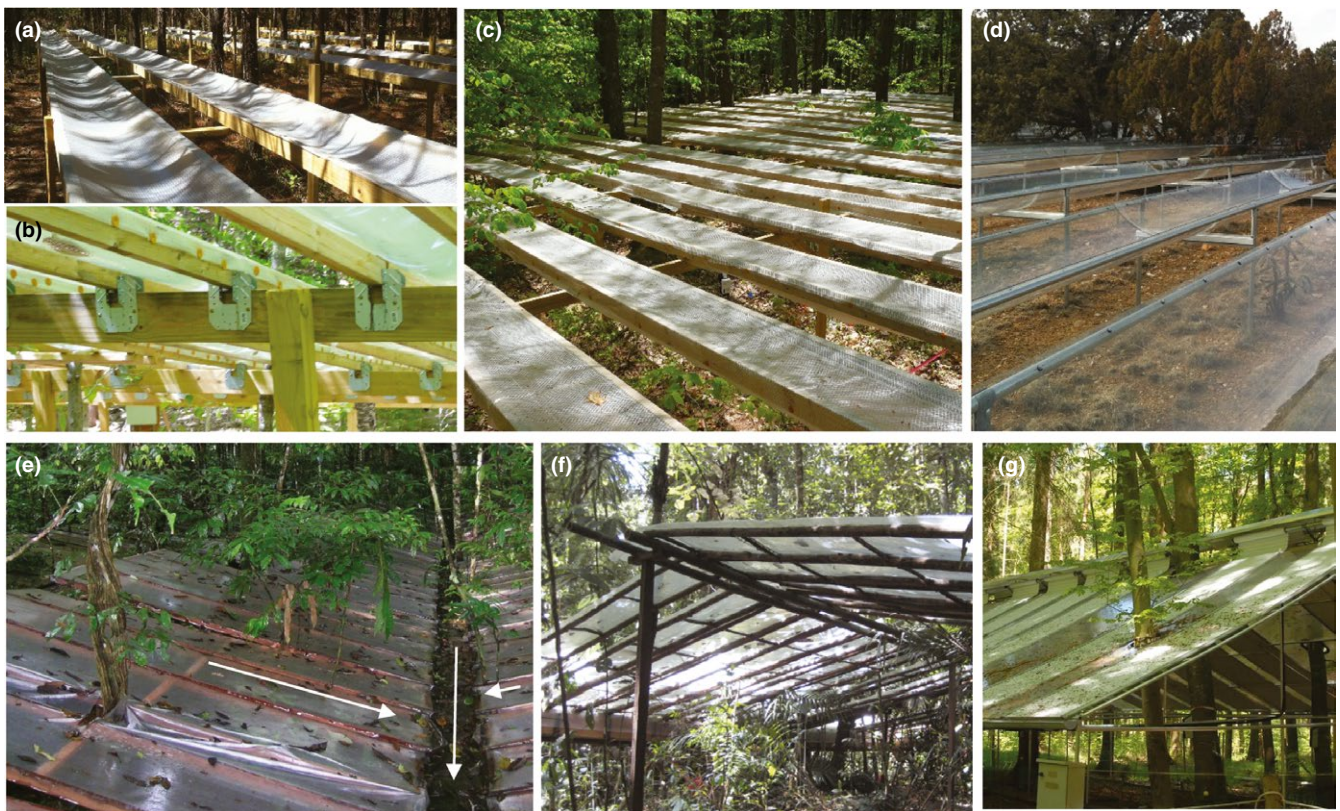
FIGURE 4 Various structural designs used to divert throughfall: (a) Fixed troughs used by the PINEMAP project (Ward et al., 2015). (b) Underside of framing braces at the Hubbard Brook LTER. (c) Fixed trough system used at Thompson Farm in Durham, NH. (d) Polycarbonate troughs and metal framing at the Sevilleta LETR (Pangle et al., 2012). (e) Flat panel system at Caxiuanã National Forest (Nepstad, 2002); arrows show the flow path from panels to a plastic-lined trough. (f) Polyethylene sheet panels at Lore Lindu National Park, Indonesia (van Straaten, Veldkamp & Corre, 2011). (g) Automated retractable roof at the KROOF project, Kranzberg Forest, Germany (Pretzsch & Schütze, 2016; Pretzsch et al., 2014). Photo credits: (a) Geoffrey Lokuta, (b, c) Cameron McIntire, (d) Aimee Classen, (e) Daniel Metcalfe, (f) Oliver van Straaten, (g) Leonhard Steinacker
