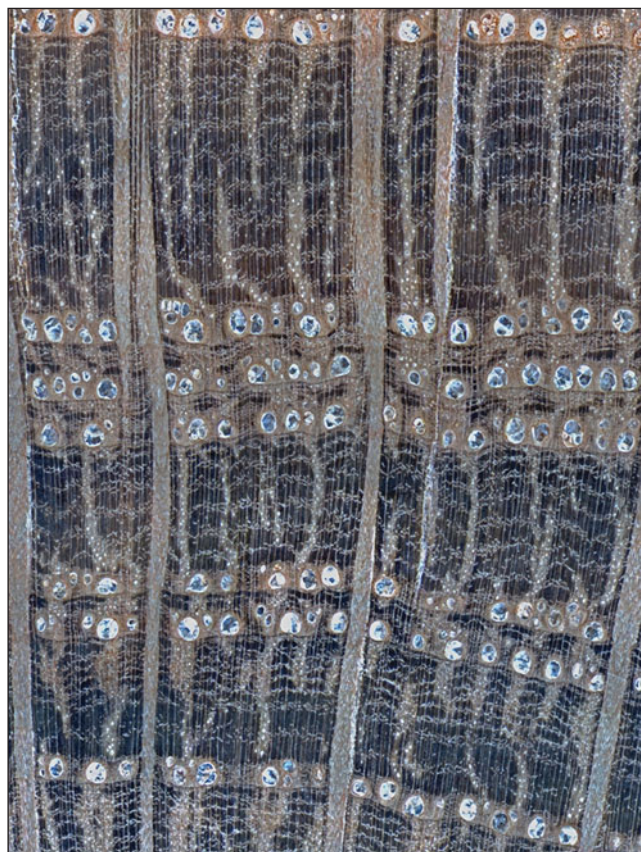
Figure 3. Microscopic view of variation in the width of six complete annual rings of white oak in southern Missouri (bark side to the top). Is average ring width a useful concept here? All graphics courtesy of the author.
