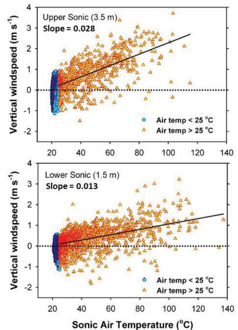
Fig. 3. The relationship between sonic air temperature and vertical windspeed measured at 10 Hz using sonic anemometers mounted at 1.5 m and 3.5 m heights above fuel beds during a fire ignited with the wind.
