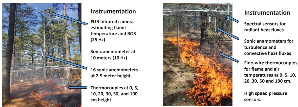
Figure 1. Instrumentation used for the 100 m<sup>2</sup> burn experiments. Four trusses were spaced approximately 2 meters apart over fuel beds. A FLIR IR camera and a single sonic anemometer were mounted at 10 m on a tower located in the middle of the plot. Sixteen sonic anemometers, radiant heat sensors, and pressure sensors were mounted in a 4 by 4 arrangement on the trusses. Thermocouple arrays were mounted every 1.2 m along the two center trusses.
