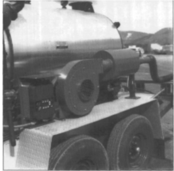
Figure 2. The electric blower adds air to regulate the temperature of the steam.
